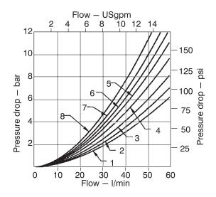
The pressure drop curves give approximate pressure drop  $\Delta P$  when passing 36 cSt (100 SUS) fluid(s) having a specific gravity. of .87.
