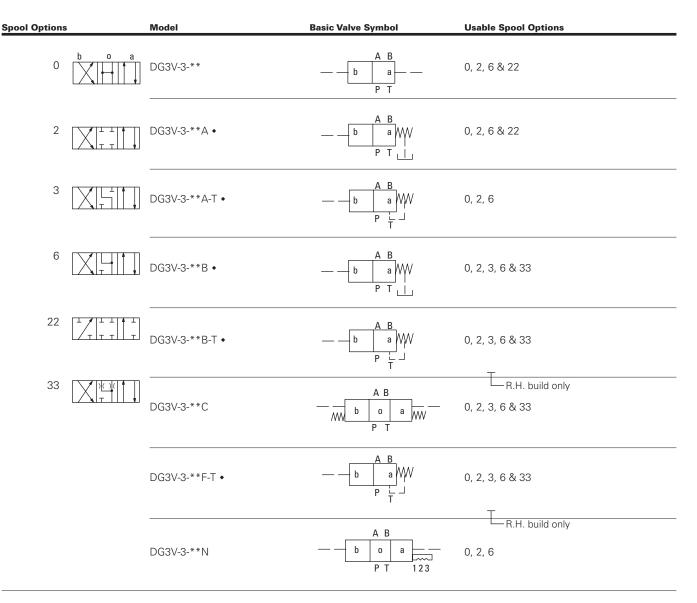
Single operator models marked • are optionally available with a manual override in the non-operator end only.
