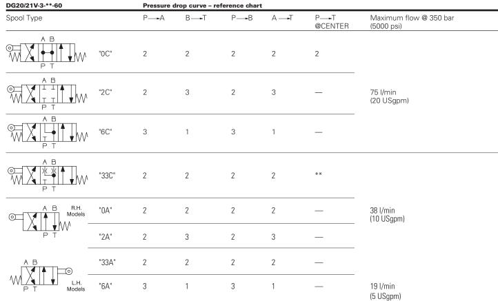
\*\*Note type "33" spool at center will pass approximately 20 I/min. (5.3 USgpm) at 124 bar (1798 psi) inlet pressure.
