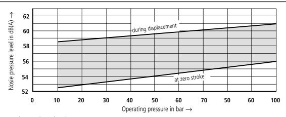
Measured in anechoic chamber to DIN 45 635, page 26
