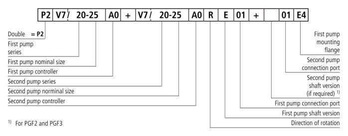
Triple and quadruple pumps are coded analogue!
