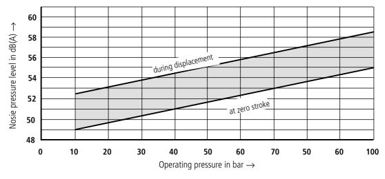
Measured in anechoic chamber to DIN 45 635, page 26
