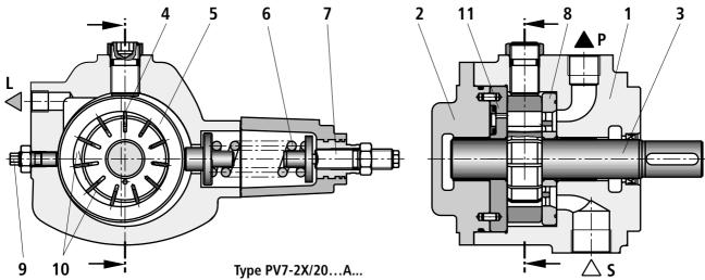
Type PV7...A hydraulic pumps are direct operated vane pumps with an adjustable displacement volume.
