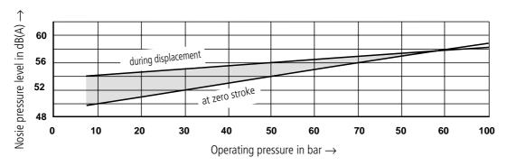
Measured in anechoic chamber to DIN 45 635, page 26
