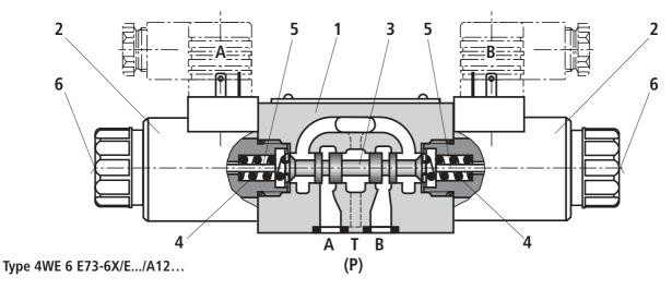
Type WE...73.. directional control valves are solenoid operated directional spool valves with soft switching characteristics. They control the start, stop and direction of flow.
