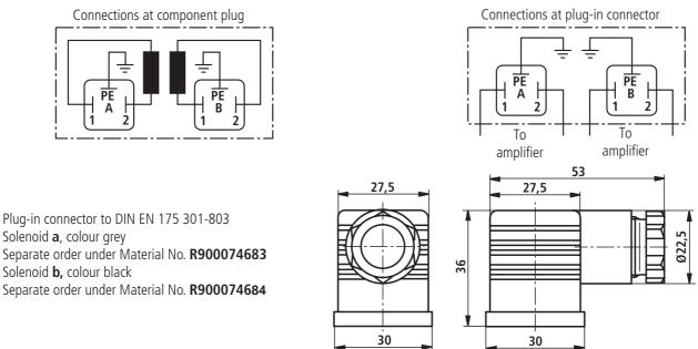
For **type 3DREPE** (with **integrated** control electronics and for version **"J"** = sea water resistant)
