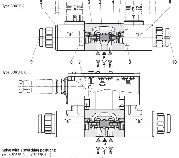
The function of this version of the valve is basically the same as that of the valve with 3 switching positions. The 2 position valves are however only fitted with either solenoid "a" (5) or solenoid "b" (6). A plug (8) is fitted in place of the second solenoid.
