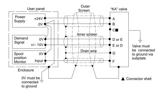
■ Spool position monitor voltage (pin F) will be referenced to the KA valve local ground. A "local ground" (pin C) is provided for optional use by differential input customer supplied electronics.
