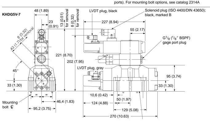
Mounting surface, seals supplied. For mating surface dimensions and subplate options, see catalog 2425. For mounting bolt options, see catalog 2314A
