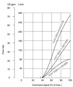
These points will vary from valve to valve, but can be adjusted using the deadband compensation feature of the drive amplifier.
